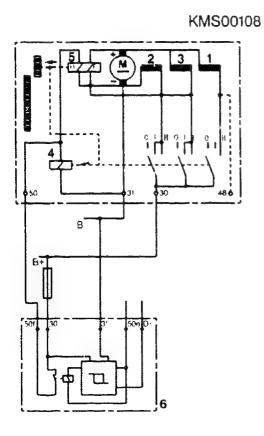
ELECTRICAL CONNECTIONS AND CIRCUIT DIAGRAMS For parallel operation of two starting motors 1 Excitation winding = 2 Shunt winding == 3 Auxiliary winding = 4 Control relay = 5 Starting-motor solenoid T Shunt winding in series with armature (as auxiliary excitation winding) Shunt winding in parallel with **IT** = armature (as speed limitation)
